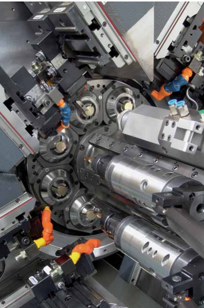
The MultiSigma's machining room. The tools are reliably monitored using ARTIS' and the processes are thus safeguarded.
