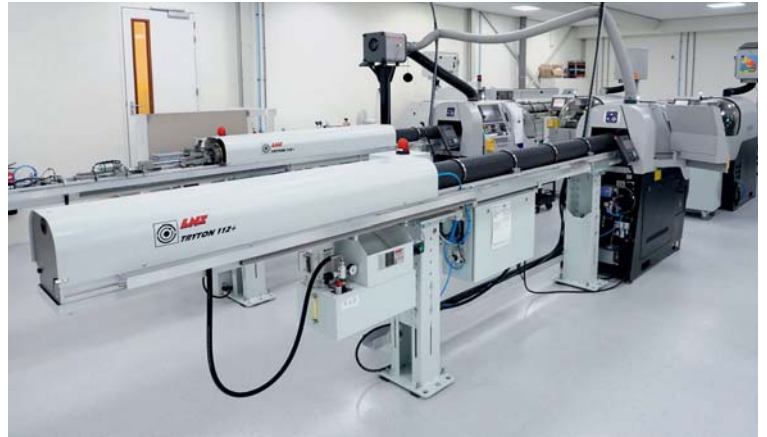
Thanks to a bar loader, Exakt Fijnmechanika can produce large series efficiently.
