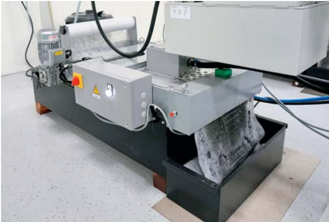
The paper belt filter system is one of the solutions that guarantees high process reliability.
