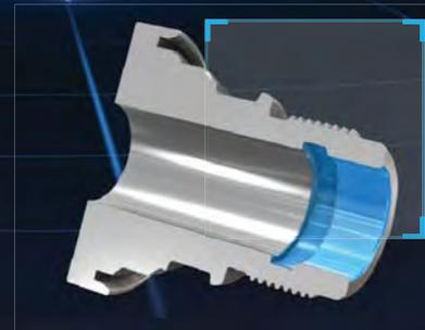
High Precision PICCO-3-CUT for Accurate Parts and Reduced Tool Stock. Coolant Through Three Sides of the Insert Directed to the Cutting Edges.
